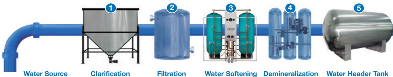
Fig. 1. Make-up Water Treatment Applications
